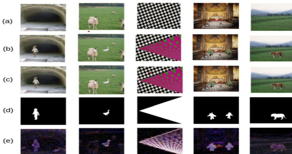
Figure 1. [1] Various sample images and their processed forms: (a) the original images (RGB colour format); (b) the images with forgery (RGB colour format); (c) the recompressed forged images (RGB colour format); (d) ground truth of forgery (Binary format); (e) difference of the tampered image with its recompressed image (RGB colour format).
